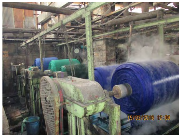
Caption: Cotton fabric dyeing using Jigger Machines
