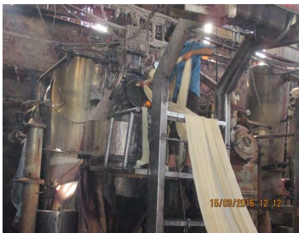
Caption: Polyester dyeing using Jet dyeing machine
