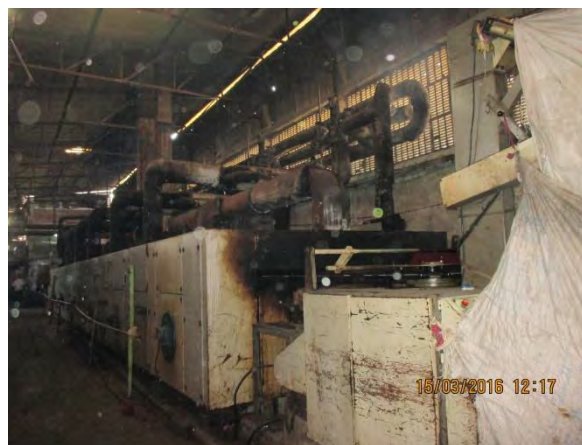
Caption: Finishing operation using Stenter
